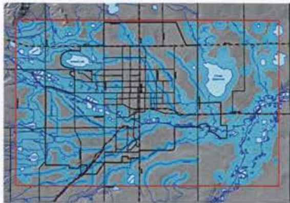
Surface Water Buffer Displayed to Detail a Varied Buffer Distance of 1/4 Mile (Small & Channelled Waterways) to 1/4 Mile (Larger Waterways, Lakes & Ponds). Single Value Assigned - 150 (High)
