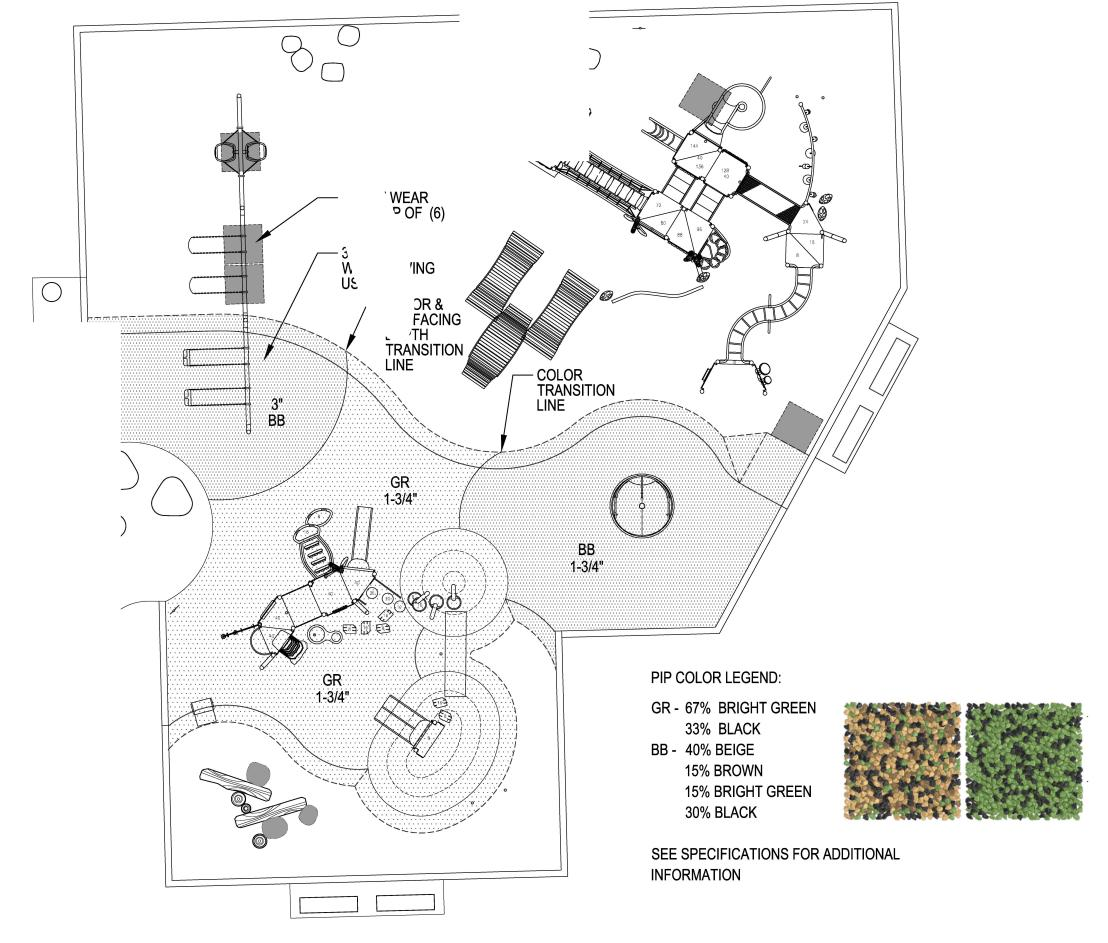
NOTE: CONTRACTOR SHALL VERIFY CRITICAL FALL HEIGHT OF PLAY EQUIPMENT WITH MANUFACTURER AND PROVIDE PLAY SURFACING TYPE AND DEPTH TO MEET ASTM-F1292
