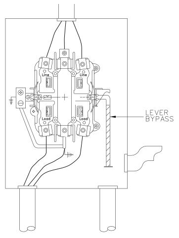
ALL NEW COMMERCIAL METERING INSTALLATIONS, REQUIRE THE INSTALLATION OF FAULT LIMITING DISCONNECTS ON THE LINE SIDE OF THE METER. THE FUSED DISCONNECT SHALL BE PURCHASED, INSTALLED AND OWNED BY THE CUSTOMER AND SHALL INCLUDE PROVISIONS FOR AN LPC SEAL. WIRE SEALS WILL BE USED BY LPC TO SECURETHE ENCLOSURE FROM UNAUTHORIZED ENTRY BUT WILL ALLOW THE CUSTOMER EMERGENCY ACCESS FOR FUSE REPLACEMENT.
